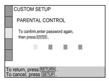
3 To confirm your password, enter it using the number buttons, then press ENTER. The display for setting the playback limitation level
